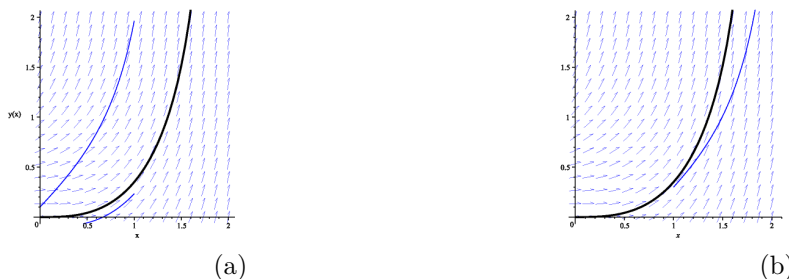
Figure 2.36: Example 2.7.5: direction field along with (a) lower and upper fences for the solution on the interval (0, 1) and (b) lower fence on the interval (1, 2) , plotted with Maple .
