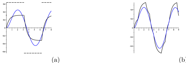
Figure 5.26: Example 5.6.3. (a) The output (black line) y_\pi(t) to the input (dashed line) and (b) output y_{\pi/4}(t) , plotted with Maple .
